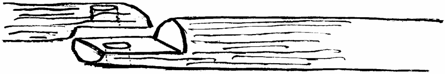
Ends of wall plates showing half lap joints
